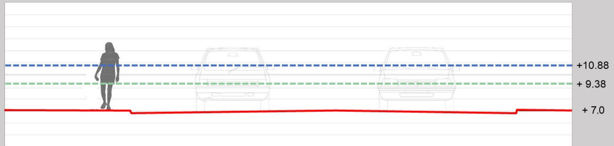
2 Day St & Concord St Flood mitigation for 1% annual storm requires a minimum of 4' additional elevation
