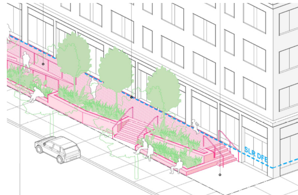
Figure 86. Flood Zoning Design Guidelines - Dry Floodproofing Source: Boston Flood Zoning Design Guidelines, Utile
